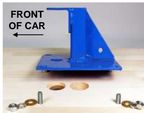
Photo # 4.2 (Brake/Steering Mount – Bolts shown for alignment only)
